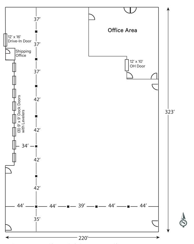
Column spacing measured from outside of column. Not guaranteed for accuracy.
