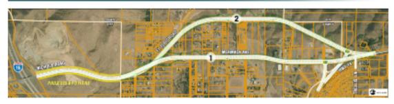
Alternative 1 consists of an alignment that follows the existing Nichols Road in Lake Elsinore and continues straight on an east-west alignment along Mermack Avenue and connects to Highway 74 north-east of Trellis Lane.
