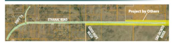
The alignment for this segment will be a direct westerly extension of the existing Ethanac Road starting from the west edge of the new San Jacinto River bridge (to be built by others), connecting to Highway 74. Three options for connecting Ethanac Road and Highway 74 are proposed to be studied in the next phase.
